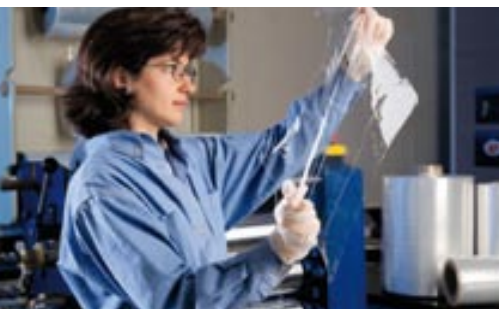
CSIRO scientist examining a transparent sheet of polymer-based material, produced for “The Breathable Film for Fresh Food” project. Image courtesy of CSIRO
