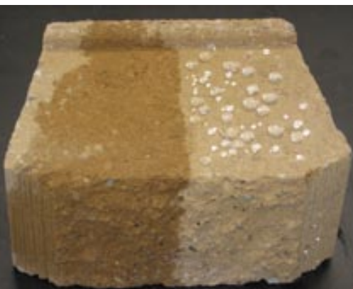
Nanoprotect® CS causing the water beading water on the stone. Image courtesy of Nanotec Pty Ltd
