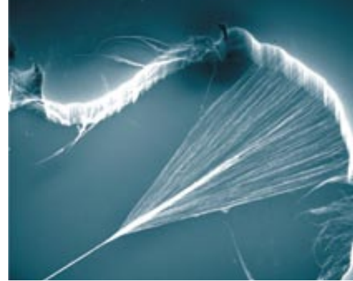
Carbon nanotubes being 'spun' to form a yarn. Image courtesy of CSIRO.
