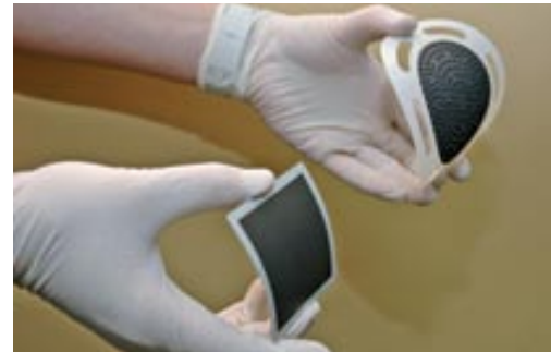
A "Ceramic Fuel Cell" - Anode and electrolyte cells. Image courtesy of Ceramic Fuel Cells.
