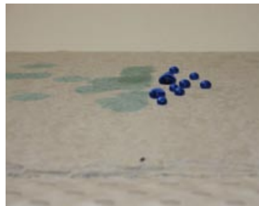
The effect of water beading after a cement sheet is treated with Nanoprotect® CS. Image courtesy of Nanotec Pty Ltd
